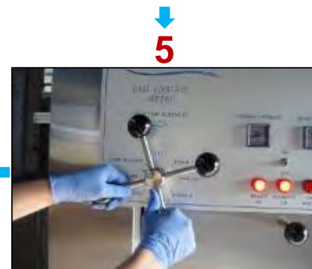
Start heating, multi-vacuum and sterilization cycles
