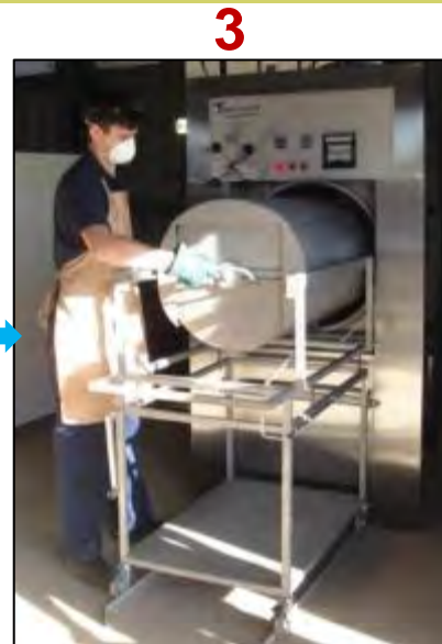
Slide barrel into autoclave
