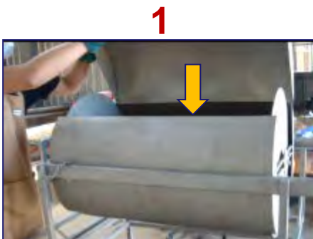
Place waste inside stainless steel barrel and close the lid
