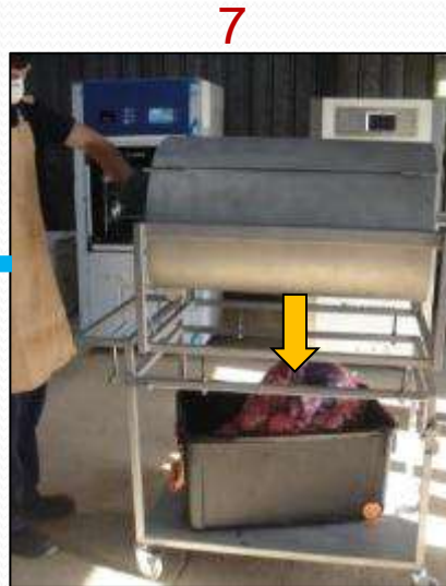
Unlock & rotate barrel to dump treated waste at the bottom
