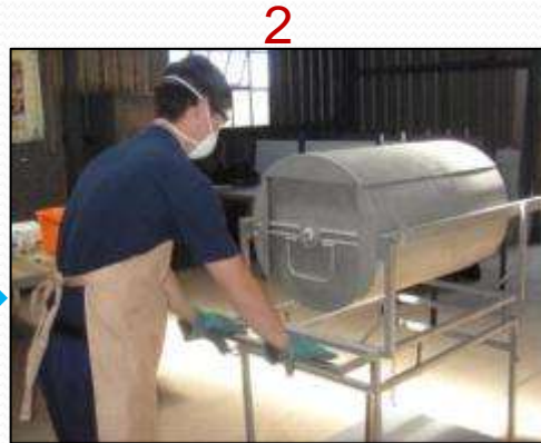
When barrel is full, take to autoclave
