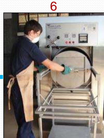
When finished, open door and remove sterilized barrel
