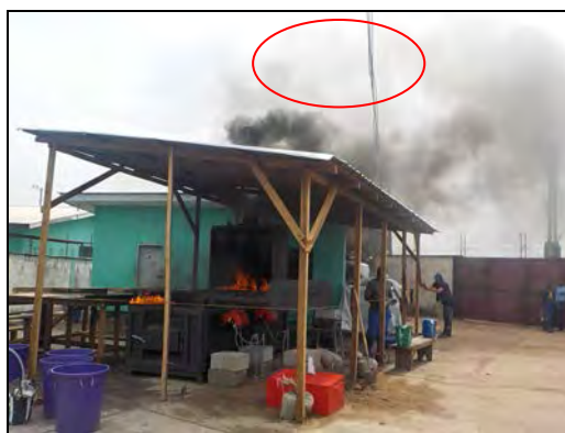
Figure 19. White haze (circled) forming after the stack indicative of HCl emissions
