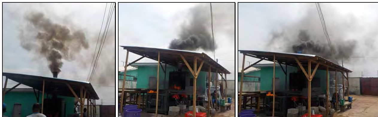
Figure 18. Heavy black incinerator smoke from the short stack of the new incinerator after addition of Ebola-contaminated waste; note fire coming out of the doors
