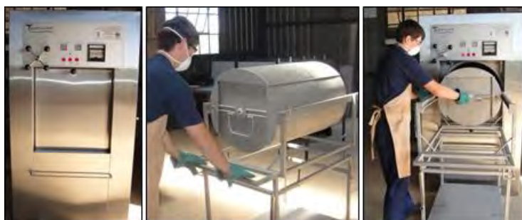
Figure 21. Medi-Clave (South Africa) autoclave sterilizer (left) and waste collection trolley with barrel
